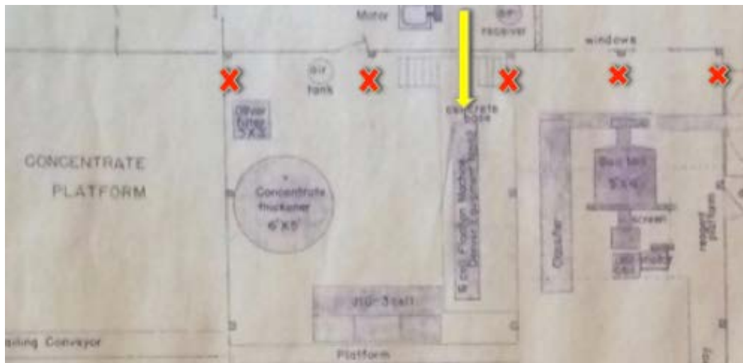
Figure 22. Red X's represent 6x6 vertical structural members, which support the walls. Yellow X represents the suspected path of the impact device or object. It is possible that an impact at this location could have destroyed or severely compromised the vertical structural members promoting early structural failure on the north end of the Mill Building, which could cause the building to lean to the north early in the event as described by Dan Sheahan.
