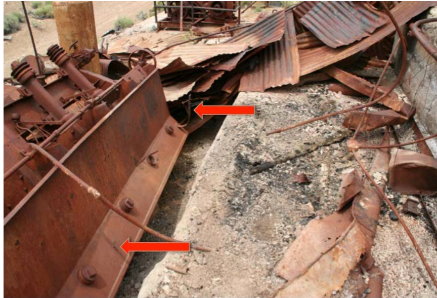
Figure 11. Top red arrows indicate one remaining strap and large wood lag bolt. Bottom red arrow indicates location of middle strap, which was torn off during dislocation of the flotation machine.
