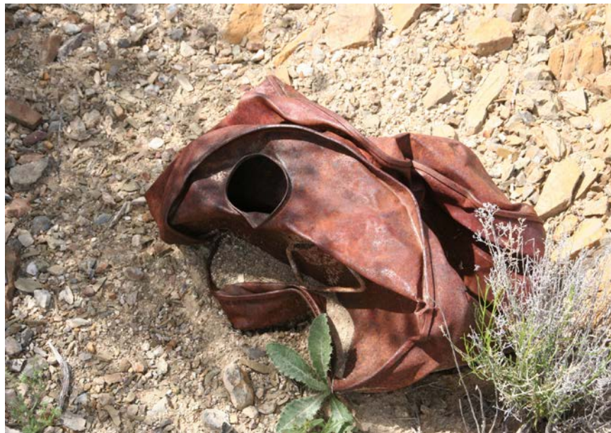
Figure 4. A metal can exhibiting effects of low-order explosive damage. This can is located south and approximately 100' from the Mill Building.
