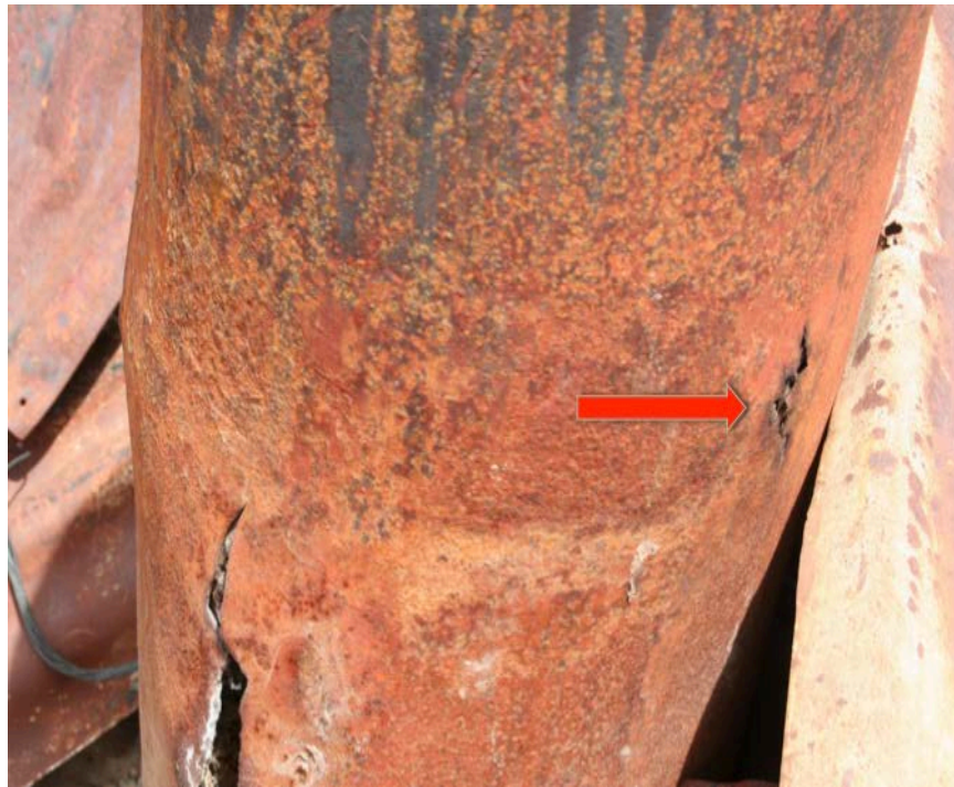
Figure 26. Third acetylene tank rupture point.
