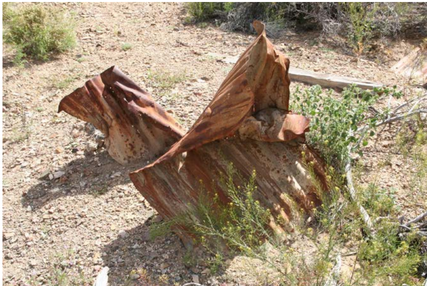
Figure 2. Roof/wall panel exhibiting effects of low-order explosive damage. This panel is located north and approximately 80' from the Mill Building.
