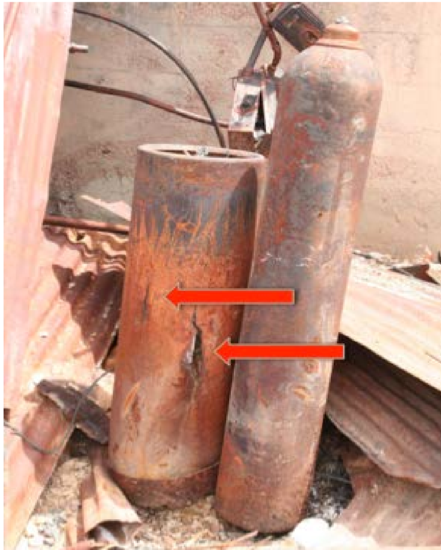
Figure 25. Acetylene tank rupture points.
