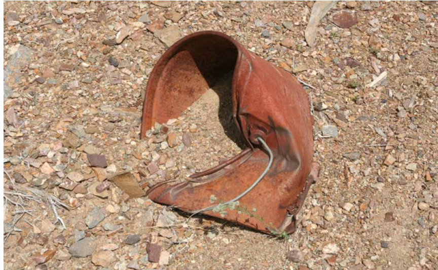
Figure 3. A metal pail exhibiting effects of low-order explosive damage. This pail is located south and approximately 130' from the building.
