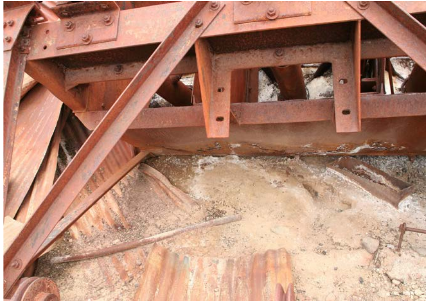
Figure 17. Roof/wall panel sandwiched underneath flotation machine. View2.
