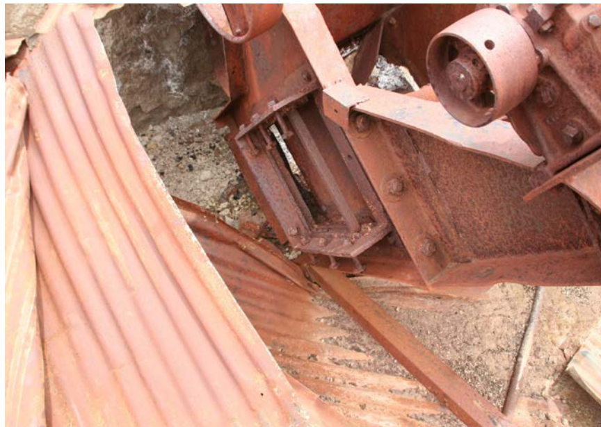
Figure 16. Roof/wall panel sandwiched underneath flotation machine. View 1.
