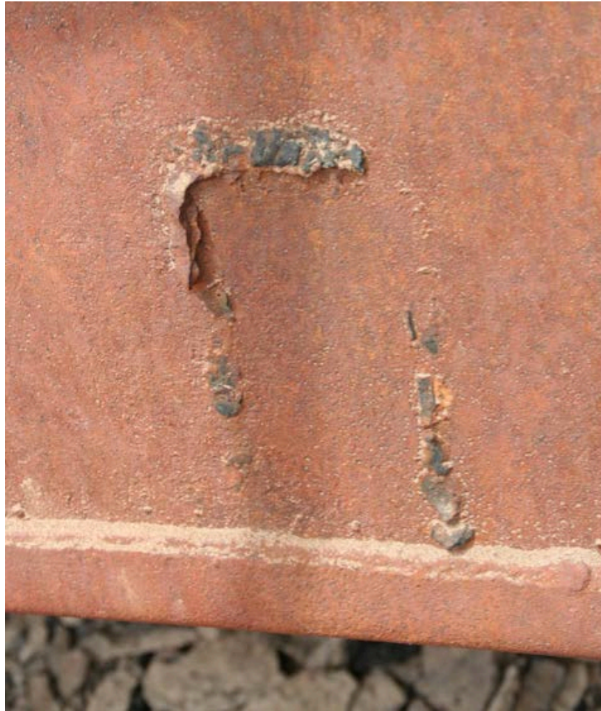
Figure 13. Attachment point of middle strap. The weld broke during the dislocation event.
