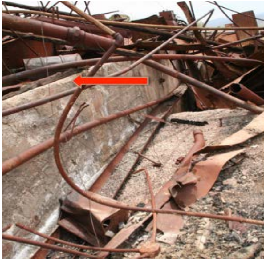
Figure 29. Small piece of frame base plate remaining on retaining wall bordering flotation machine terrace. Mass loss due to exposure to fire is greater nearer the point of entry of suspected impact object.
