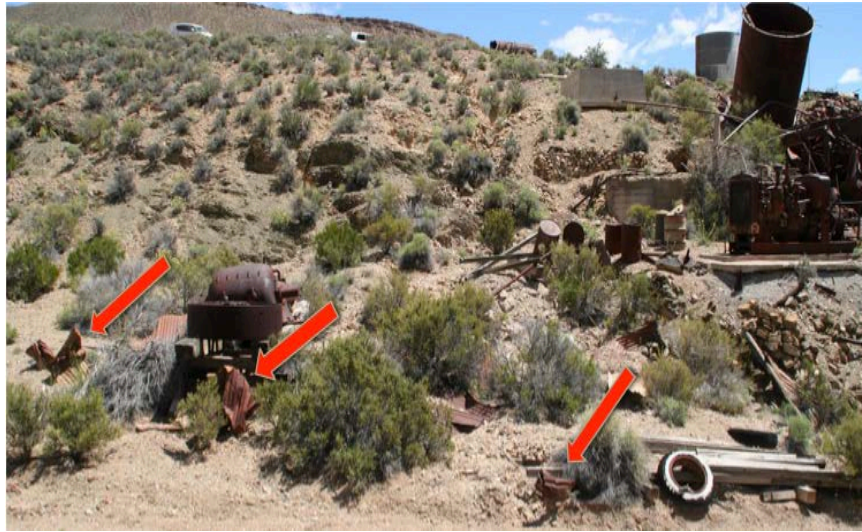
Figure 1. Corrugated metal roof/wall panels exhibiting low-order explosive damage. These panels are located to the north of the Mill Building and are approximately 50-70' from the building.
